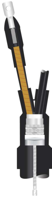
1.1 kV PILC Termination
